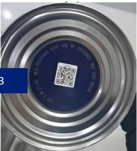
QR code 3 on the bottom stuck during production
